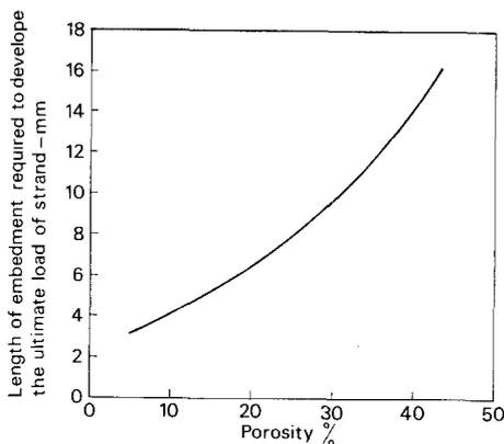
Figure 2 Relation between porosity of matrix and the critical length of embedment required to develop the ultimate load in the strand.
