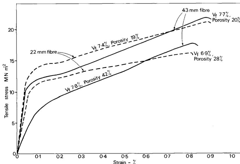
Figure 7 Stress–strain relation in tension of grg composites for two fibre lengths having different porosities.
