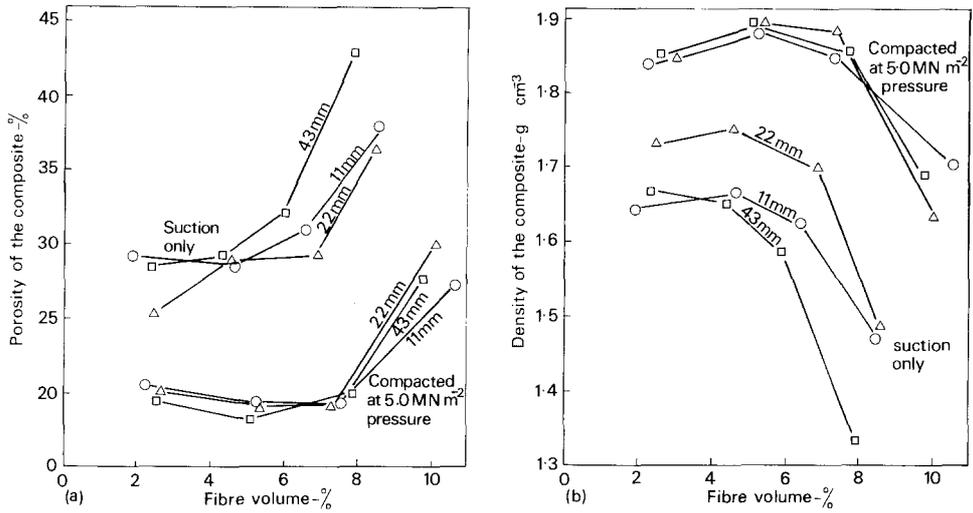
Figure 3 Relation between fibre content, porosity and density of grg composites made by spray-suction technique.
