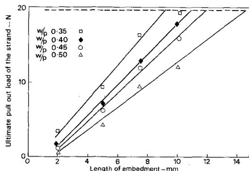
Figure 1 Relation between ultimate pull-out load and length of embedment of "E" glass strand in plaster of paris.
