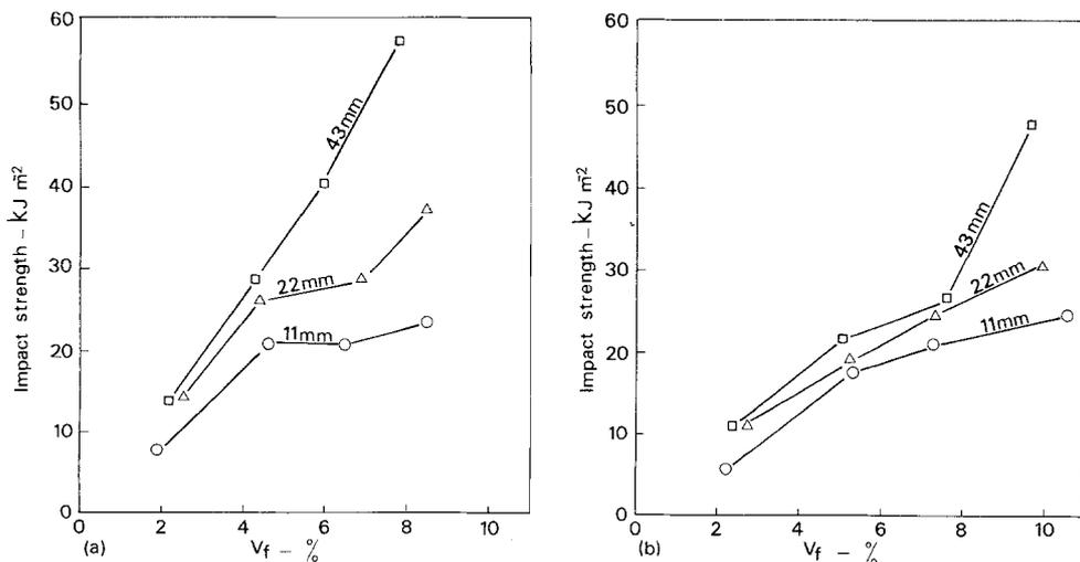
Figure 6 Relation between impact strength and fibre content of grg composites for different fibre length made by (a) spray-suction only, (b) spray-suction and compacted at  $5.0 \text{ MN m}^{-2}$  pressure.
