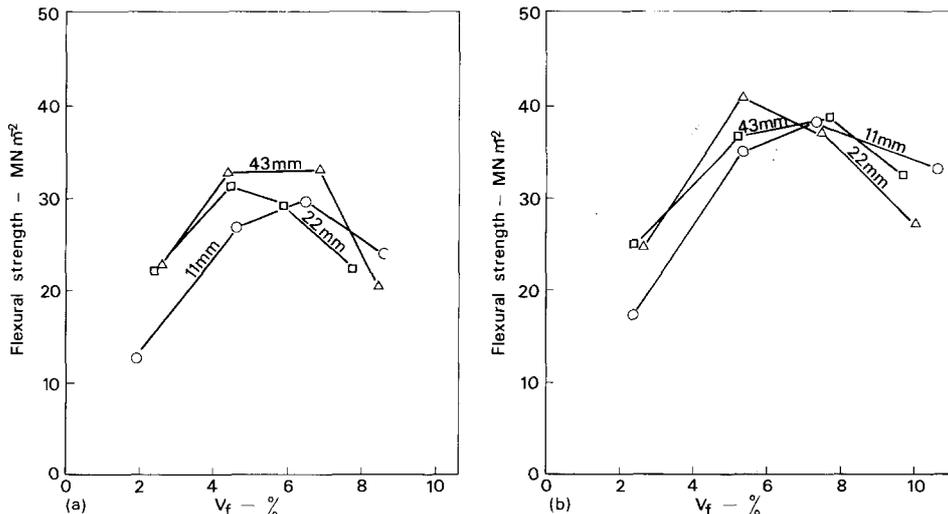
Figure 4 Relation between flexural strength and fibre content of grg composites for different fibre lengths, and made by (a) spray suction only, (b) spray suction and compacted at  $5.0 \text{ MN m}^{-2}$  pressure.
