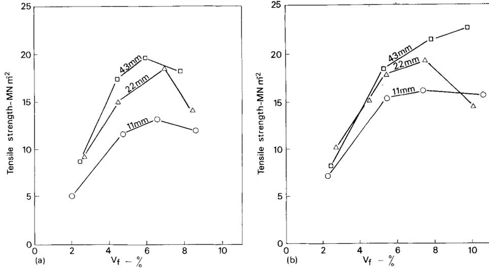
Figure 5 Relation between tensile strength and fibre content of grg composites for different fibre lengths and made by (a) spray-suction only, (b) spray-suction and compacted at  $5.0 \text{ MN m}^{-2}$  pressure.
